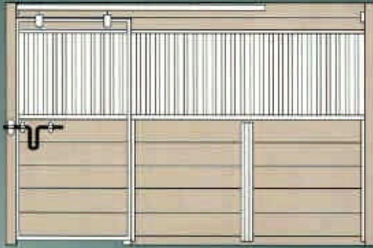
Package 4650 Stall Front with Grill in Front and Slide Door Shown with Optional 4901 Track and Hardware
